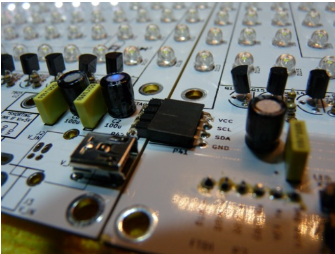
Joining the two boards together - can you spot the 'drunk' transistors?
